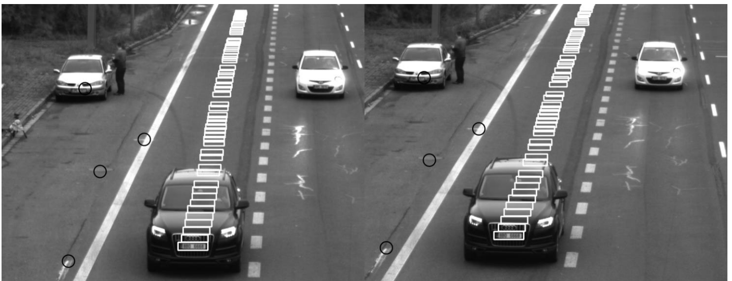
Figure1: Left and right camera images with license plate detector output and highlighted calibration points.
