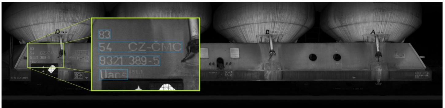
Figure 1: Input image example of a goods wagon with highlighted label box (green) and individual textboxes (blue).
